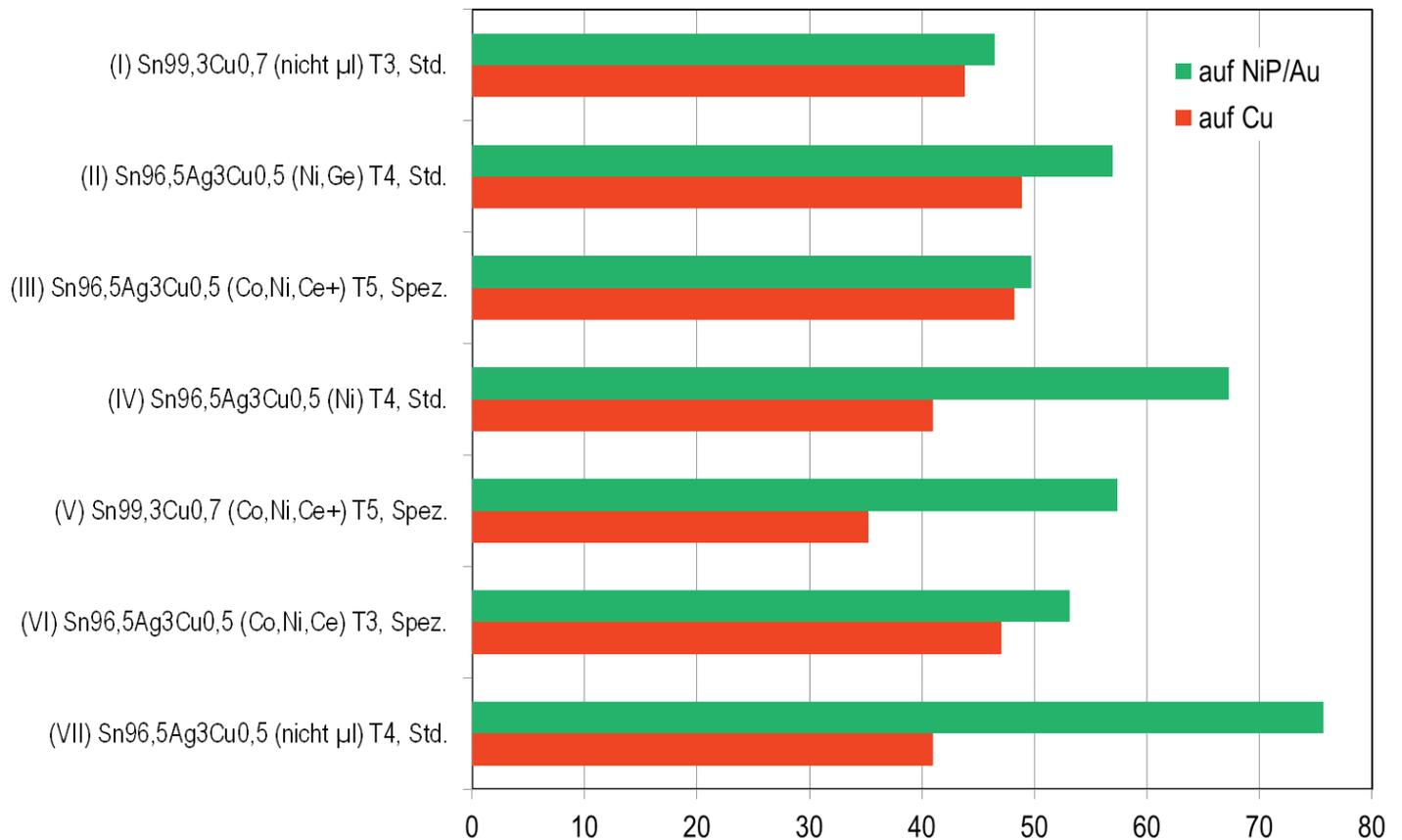
Fig. 4: Shear strengths after 1000 temperature cycles
