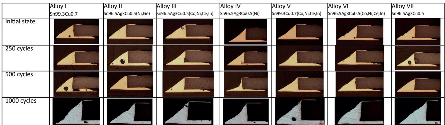
Fig. 5: Microsections on Cu PCB
