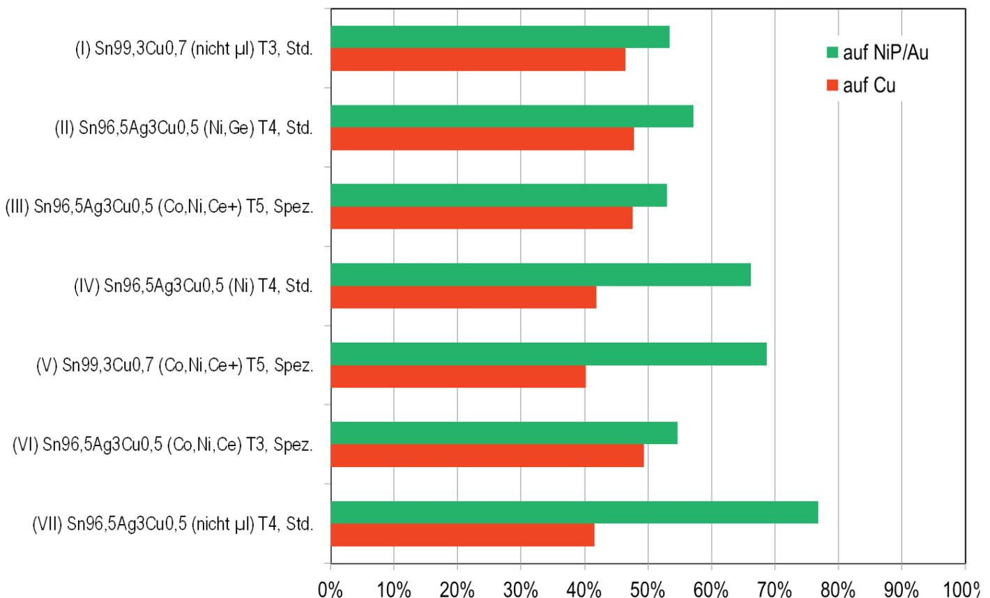
Fig. 8: Standardised shear forces after 1000 temperature cycles
